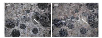
In a self-healing bioconcrete, dormant bacterial spores contained in clay pellets (black and gray circles, left) germinate when cracks expose them to moisture. The microbes feed on calcium lactate to form limestone, sealing the cracks (right). Credit: Delft University of Technology.
